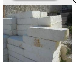
• Kayseri stone is darker in color than stone traditionally used in Cappadocia, but it is very strong and water-tight. Therefore it is good to use this stone for foundations and exterior stairs & also to top parapet walls.
